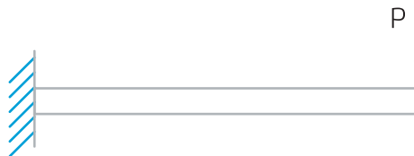
Figure 10. Cantilever beam with a point-applied end load
