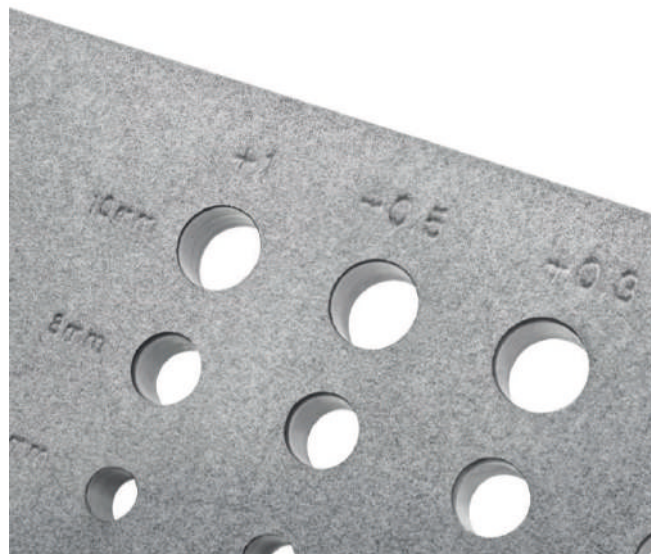
Figure 2: HP MJF pre-formed hole testing
