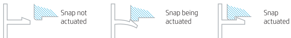
Figure 2. Cantilever snap-fit assembly operation
