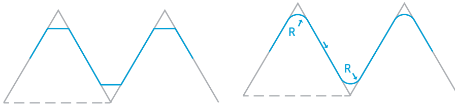
Figure 5: Round edges for custom-printed threads
