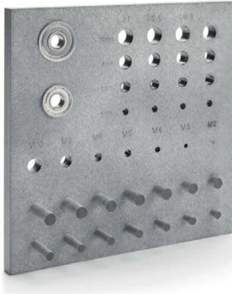
Figure 3: Bearings inserted into an HP MJF part
