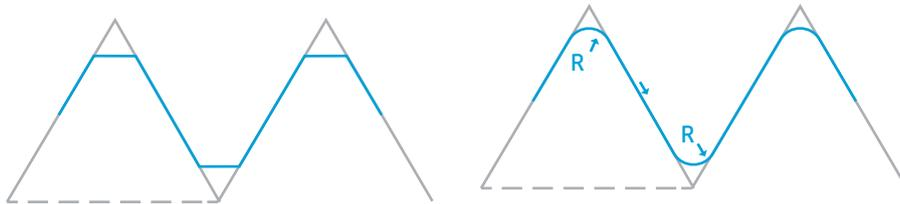
Figure 5: Round edges for custom-printed threads
