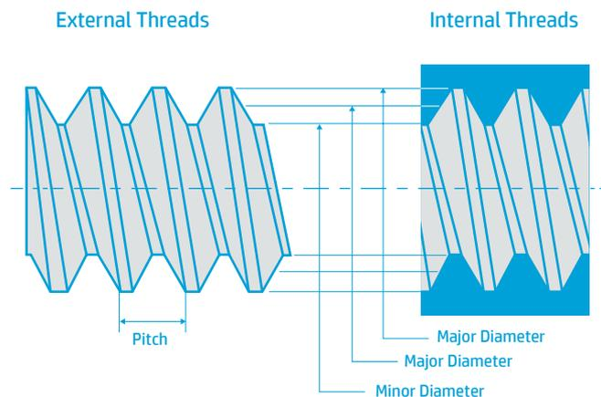
Figure 4: Features of external and internal threads
