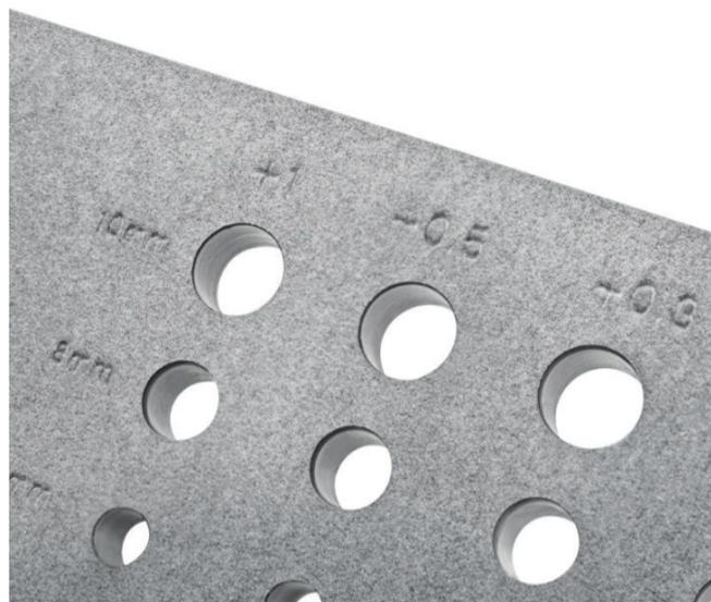
Figure 2: HP MJF pre-formed hole testing
