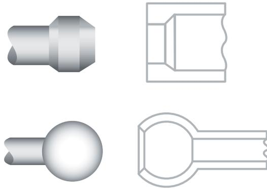
Figure 7. Annular snap-fit
