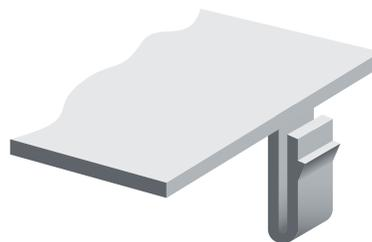
Figure 5. U-shaped snap-fit
