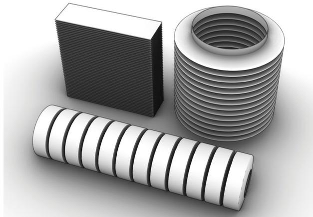
*Figure 10: Recommended print orientation for sample designs*
