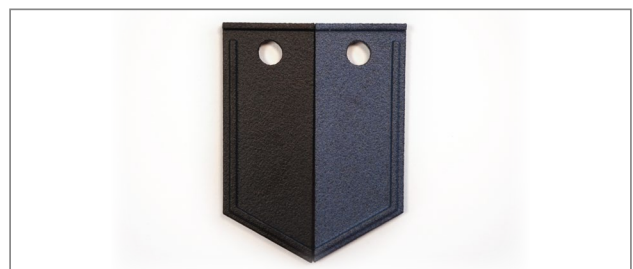
Figure 24: Textile dye on HP 3D HR PA 12 (PSS) before vs. after lightfastness testing
