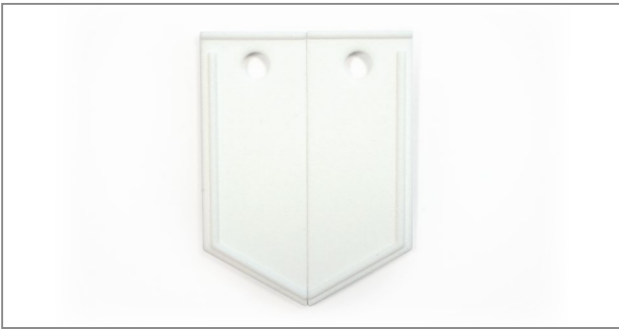
Figure 14: Raw, unfinished EOS PA 2200 sample
