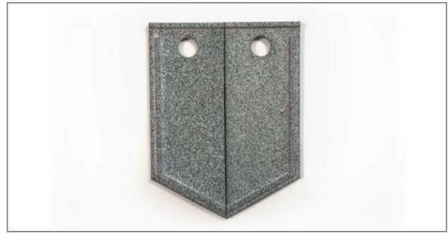
Figure 15: Raw, unfinished HP 3D HR PA 12 sample
