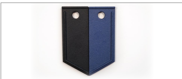
Figure 22: Textile dye on EOS PA 2200 (PSS) before vs. after lightfastness testing
