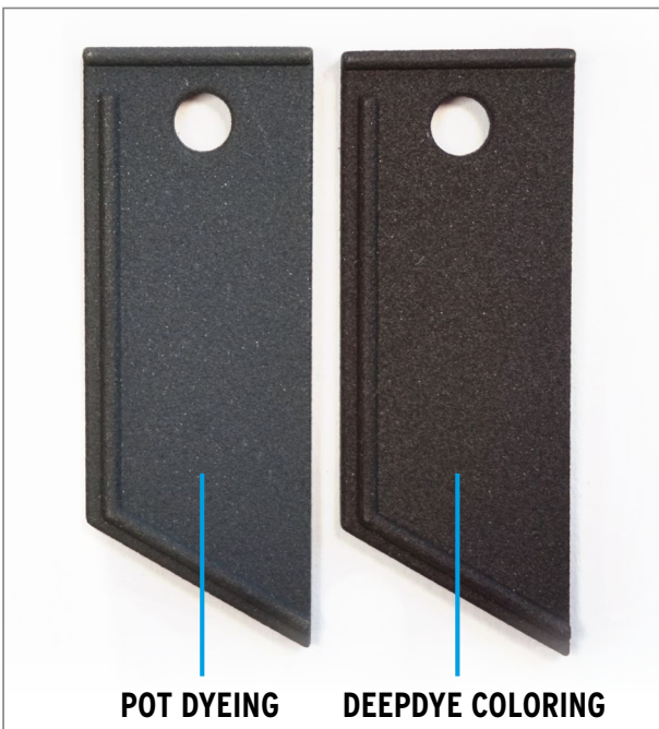
Figure 16: EOS PA 2200 sample part after dyeing with textile dye and DM Black 01 - parameters see table 2
