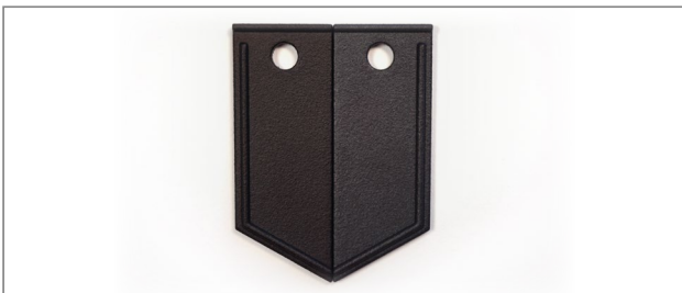
Figure 21: DM Black 01 on EOS PA 2200 (PSS) before vs. after lightfastness testing
