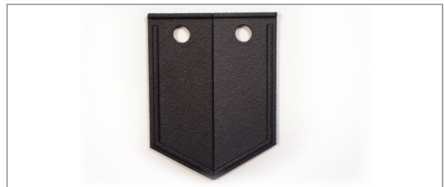
Figure 23: DM Black 01 on HP 3D HR PA 12 (PSS) before vs. after lightfastness testing
