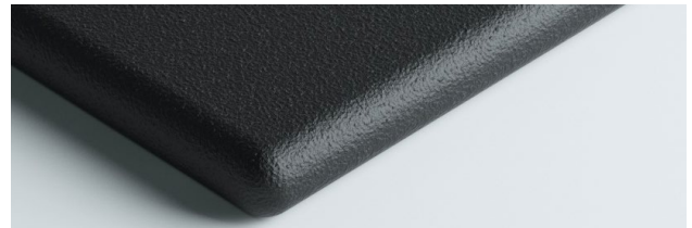
Figure 19 & 20 LTR: Visualization of a HP 3D HR PA 12 sample dyed with DDC without surface treatment and a part treated with PolyShot Surfacing (PSS) before dyeing
