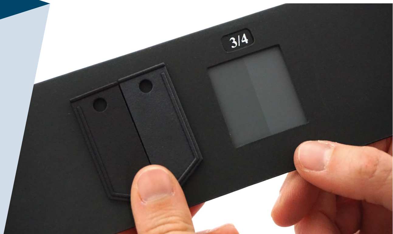
Figure 18: Visual comparison of a sample part (before and after the test) with the grey scale
