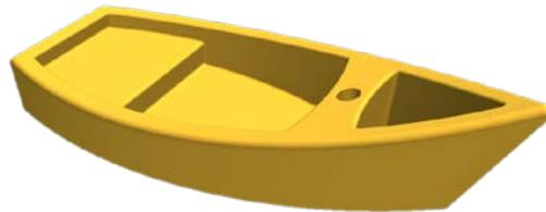
The visible area of the final part will be the top of it, therefore this area must be placed face down in order to increase smoothness:
