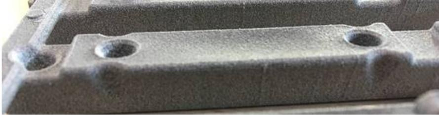
For parts that are thick and dense you might experience a local shrinkage on the surface of the part. This is more frequent on top surfaces.
