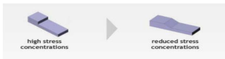
*Reducing the stress concentration in the transition of the sections with different thicknesses*
