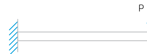
Figure 10. Cantilever beam with a point-applied end load
