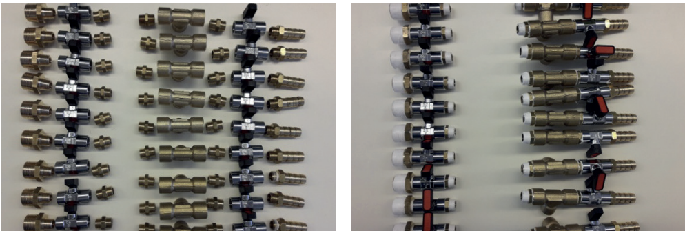
Connectors used for the tightness tests
